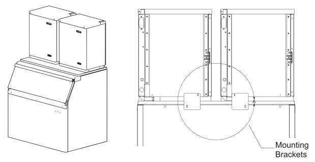
6. Secure ice machine heads to the adapter and the bin using one mounting bracket each. Use the supplied brackets and hardware.
